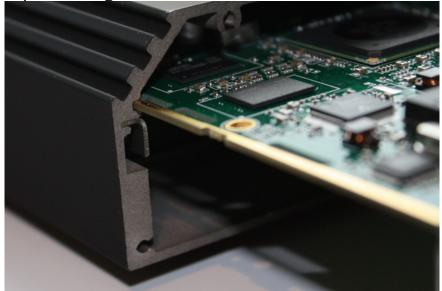
9. Mount the back side piece with the three screws. Be careful when inserting the screws, making sure that the threads are aligned correctly.
