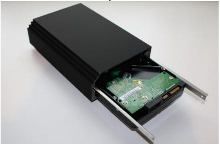
7. Slide the circuit board into B3 above the hard drive.
